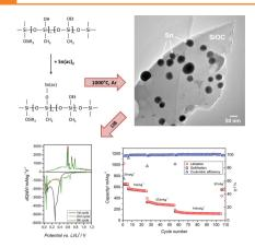
Enhanced lithium storage stability of single-source precursor-derived SiOC/ Sn nanocomposites is demonstrated. The nanocomposites comprise an amorphous SiOC matrix and in-situ formed Sn precipitates. Capacity measurements outline different final Li-Sn alloy stages, depending on the matrix. Galvanostatic cycling shows a first cycle reversible capacity of 566 mAhg-1 for SiOCMK/Sn and 651 mAhg<sup>-1</sup> for SiOCRD/Sn.
