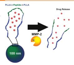
Triblock copolymer nanoparticle with tunable drug release. Nanocarriers based on PLLA-b-peptide-b-PLLA copolymers are proved to have exceptional material properties for controlled drug release in response to MMP-2-dependent peptide cleavage. Comparison specimens demonstrate the tunable bioactivity of these nanocarriers based on polymer constitution. As MMP-2 is selectively overexpressed in tumor tissues, this is a promising system for solid tumor cancer therapy.
