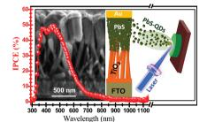
Pulsed laser deposition (PLD) is advantageously used to decorate TiO2-nano rods (TiO2-NRs) with PbS-quantum dots (PbS-QDs) to achieve highly efficient nanohybrid-heterojunctions (NH-HJ) solar cells. By optimizing the characteristics of both PLD-deposited PbS-QDs and TiO2-NRs, while introducing MoO<sub>3</sub> hole extracting layer and single-wall carbon nanotubes efficient charge carrier, NH-HJ PV-devices exhibit power conversion efficiencies as high as 5.3% (under AM1.5 solar illumination).
