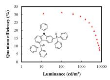
Excellent thermal stability and high quantum efficiency above 30% in blue phosphorescent organic light emitting diodes are achieved using a high triplet energy host material with two electron withdrawing substituents at asymmetric positions of carbazole.
